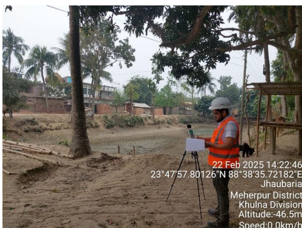
Figure-10: Ambient Noise level measuring in the field at day time.
