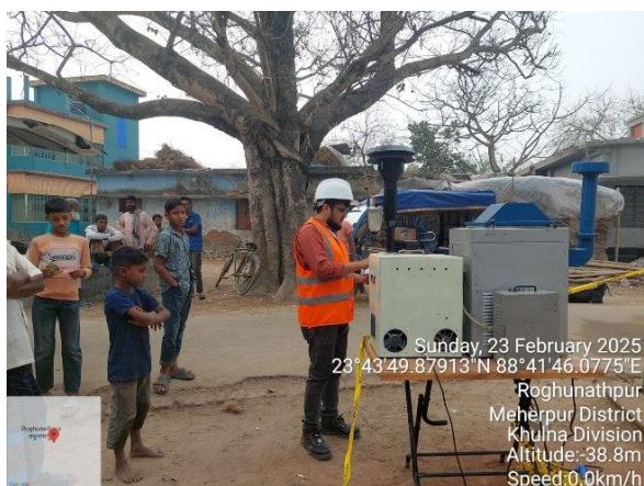
Figure-12: Ambient Air Quality Sampling in The Project Area
