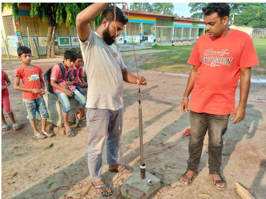
Figure 8: Slug Test in a Monitoring Well
