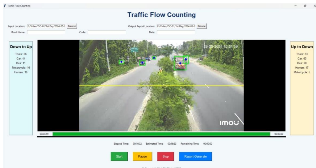
Figure 4-9: Digital Video Traffic Counting Using Software
