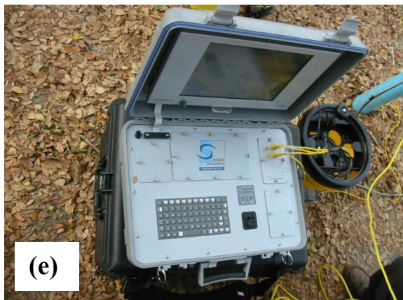
Figure 8 (a) Freedom Data PC with P-SV Downhole Source and 1 Tri-axial Geophone Receiver used in Crosshole Seismic Investigations; (b) Main Component of the Freedom Data PC; (c) Impact directions which are on the left, right and vertical directions; (d) Triaxial geophone behavior; (e) computer with cables which are connected to the geophone; (f) Field Data Acquisition by PS logger.
