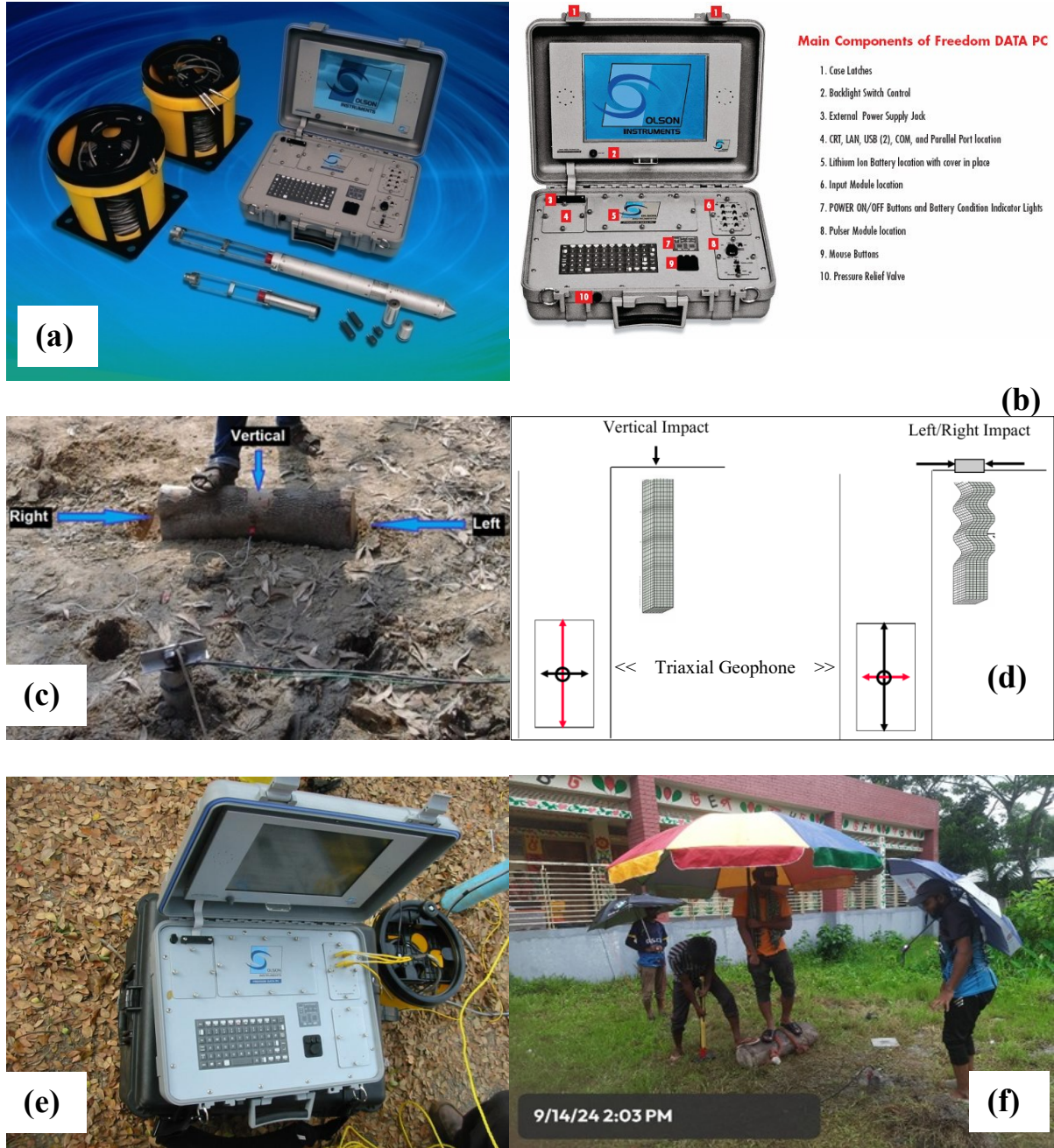
Figure 7 (a) Freedom Data PC with P-SV Downhole Source and 1 Tri-axial Geophone Receiver used in Cross hole Seismic Investigations; (b) Main Component of the Freedom Data PC; (c) Impact directions which are on the left, right and vertical directions; (d) Triaxial geophone behavior; (e) computer with cables which are connected to the geophone; (f) Field Data Acquisition by PS-logger.
