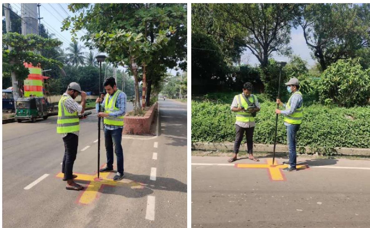
Figure 5-3: GCPs value collection for drone survey by RTK GPS
