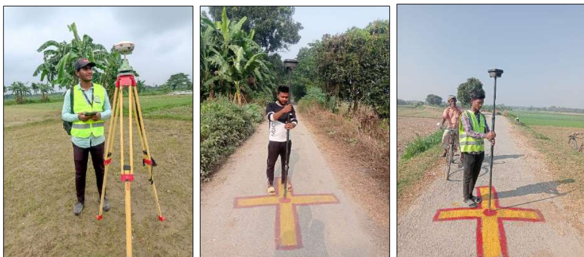
Figure 3-5: GCP Value Collection for UAV Image Capturing
