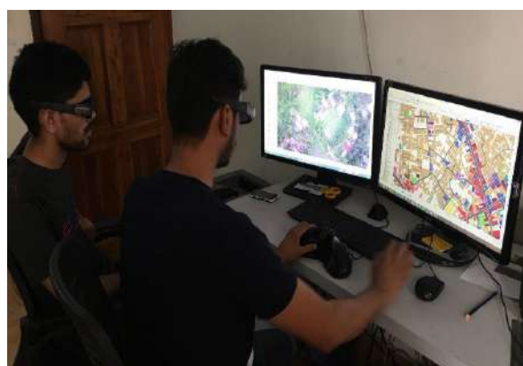
Figure 4-1: 3D Feature Extraction from stereo model using photogrammetric method
