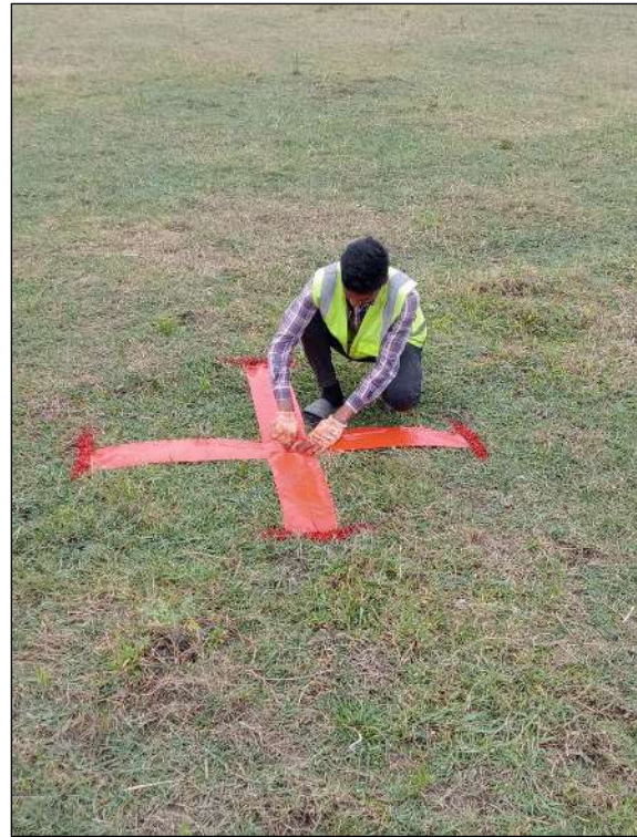
Figure 3-4: GCP Marking on Ground As per GCP Plan Before Drone Survey
